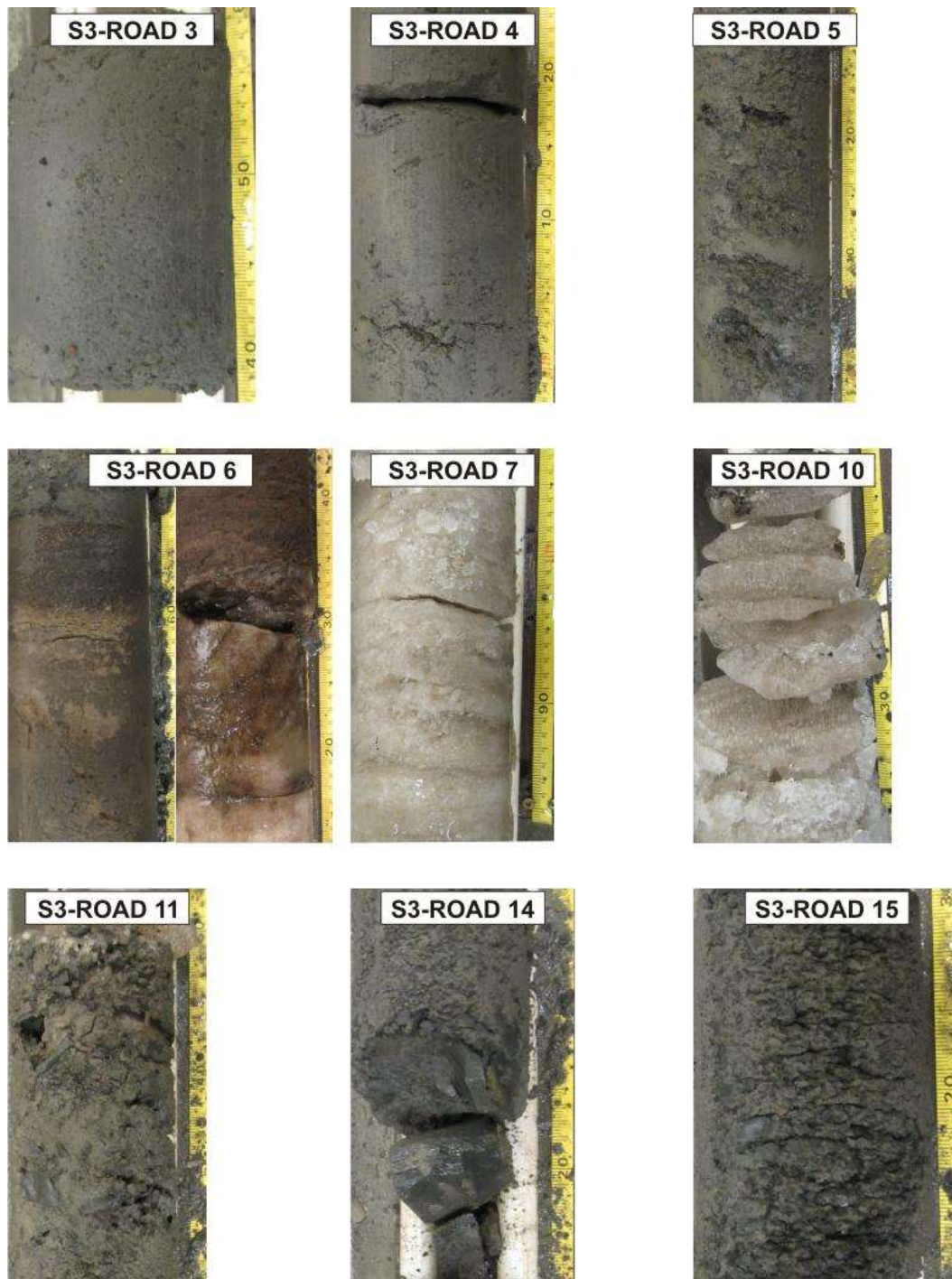
Permafrost features for Site 3 under the road.
