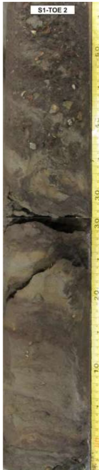
Permafrost features for Site 1 under the toe of the Embankment.
