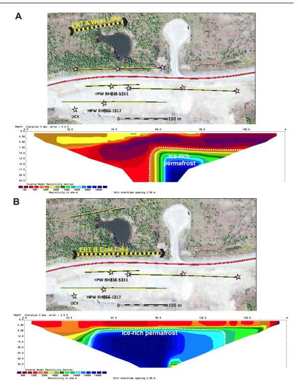
Figure 4.2.6. ERT Surveys performed at Dry Creek rest area site for A) West of the thermokarst lake; and B) East of the thermokarst lake.
