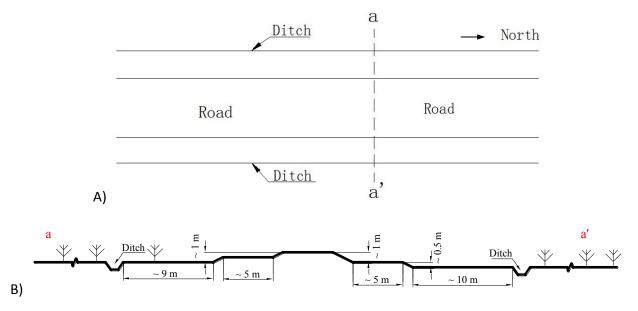
Figure 4.3.7. Schematic illustration of the Enger Creek adaptation site for A) Localisation of proposed embankment cross section and transverse profile; and B) a-a' embankment cross section at km 1863.5.
