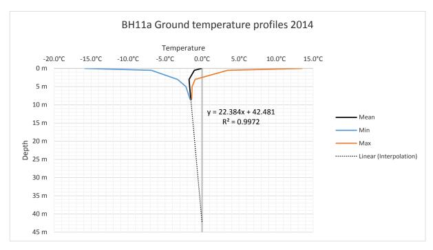
Figure 4.5.9. Interpolation of the permafrost base at BH11a
