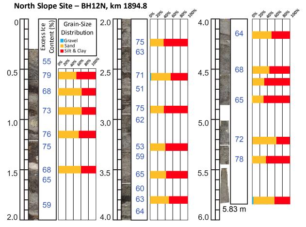
Figure 4.6.4. Log of borehole BH12N.
