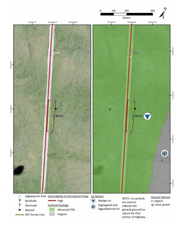
Figure 4.3.1. Vulnerability maps of Site 3 (satellite imagery and surficial geology) 66
