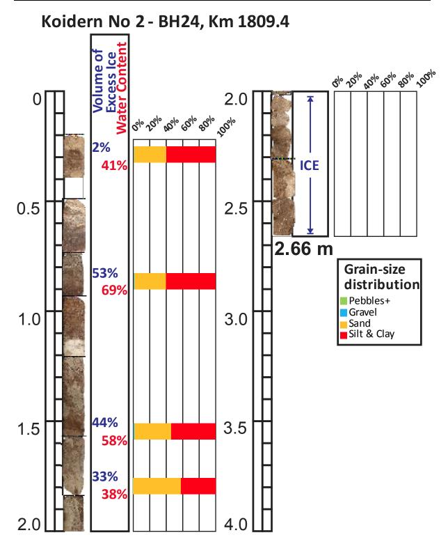
Figure 4.1.2. Log of borehole BH24.
