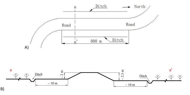
Figure 4.4.9. Schematic illustration of the field site A) Localisation of proposed embankment cross section in transverse profile; and B) a-a' embankment cross section km 1896.3
