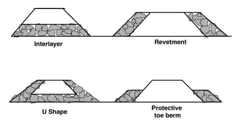
Figure 3.3. Various ACE embankment configurations
