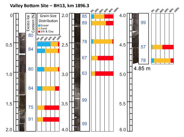
Figure 4.4.2. Log of borehole BH13.
