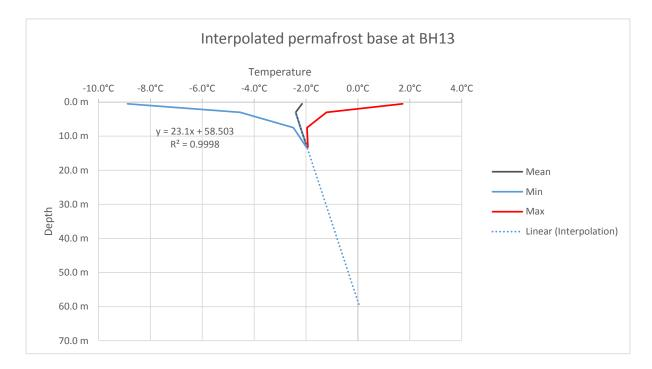
Figure 4.4.8. Interpolation of the permafrost base at BH13.
