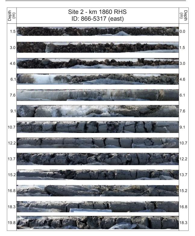
Figure 4.2.5. Cores collected from borehole HPW 866-5317 (east).
