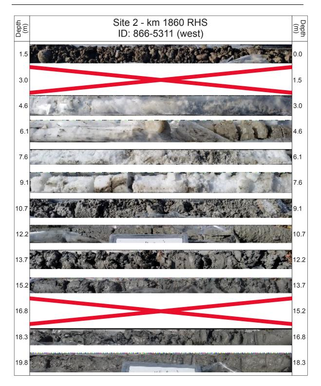
Figure 4.2.3. Core collected from borehole HPW 866-5311 (west).
