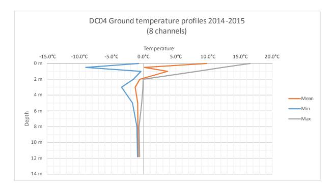
Figure 4.2.9. Ground temperature recorded in DC4 from November 2014 to October 2015 including 8channels data.
