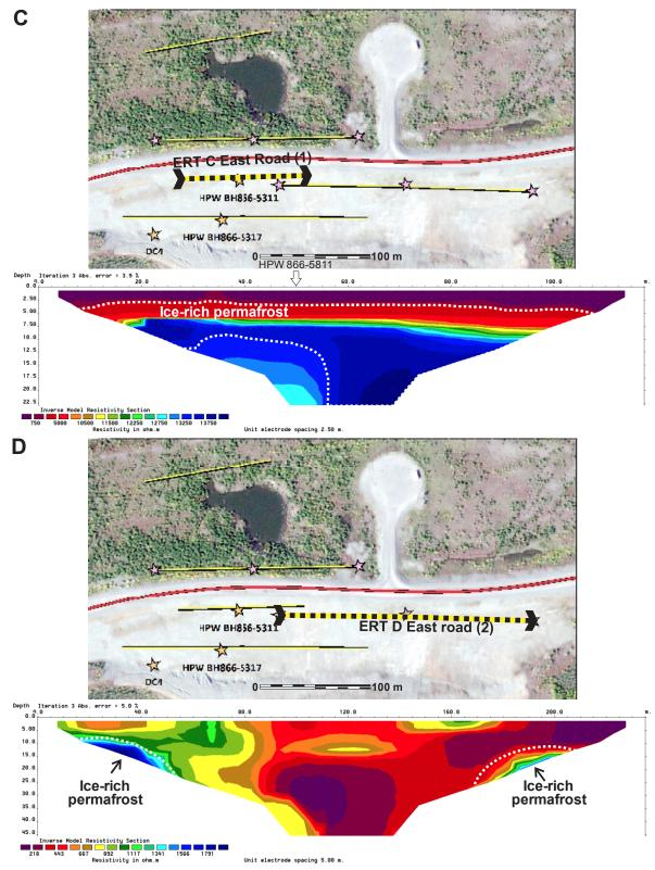
Figure 4.2.6 (cont.). ERT Surveys performed at Dry Creek rest area site for C) East of the road (North); and D) East of the Road (South). 54
