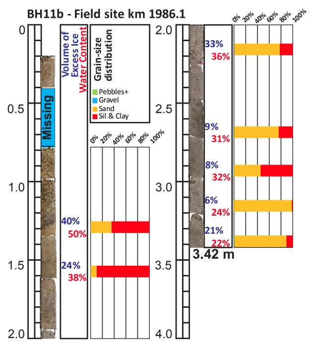
Figure 4.5.3. Log of borehole BH11b.
