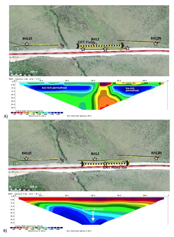
Figure 4.6.7. ERT Surveys performed at borehole BH12 for A) the field; and B) the toe of the highway embankment.
