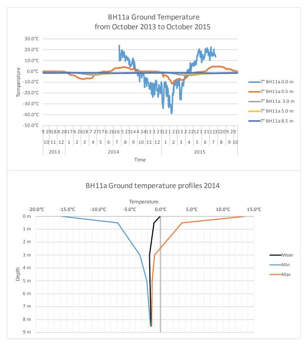
Figure 4.5.7. Ground temperature recorded in BH11a from October 2013 to October 2015.
