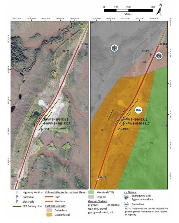
Figure 4.2.1. Vulnerability maps of Site 2 (satellite imagery and surficial geology)
