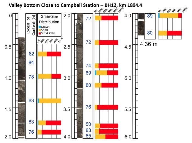
Figure 4.6.2. Log of BH12 borehole.
