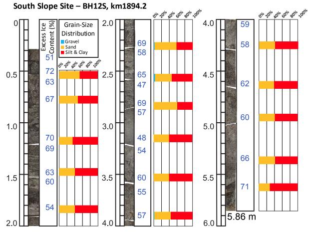
Figure 4.6.3. Log of borehole BH12S.
